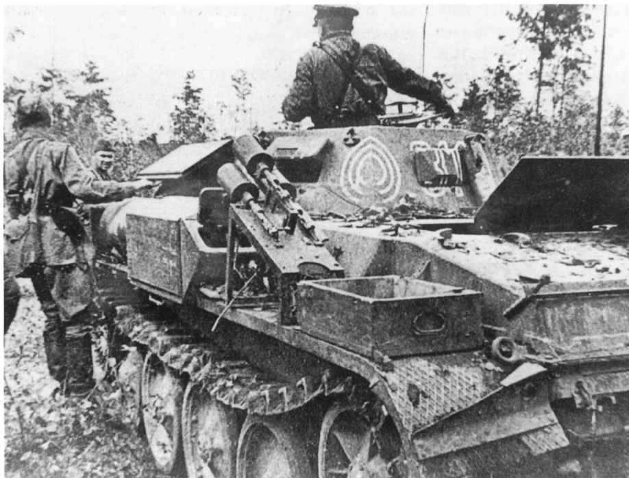
A Panzerkampfwagen II (F) converted from a Panzerkampfwagen II Ausf.E, which had lubricated bearing tracks. This Flammpanzer was captured by Russian forces.
