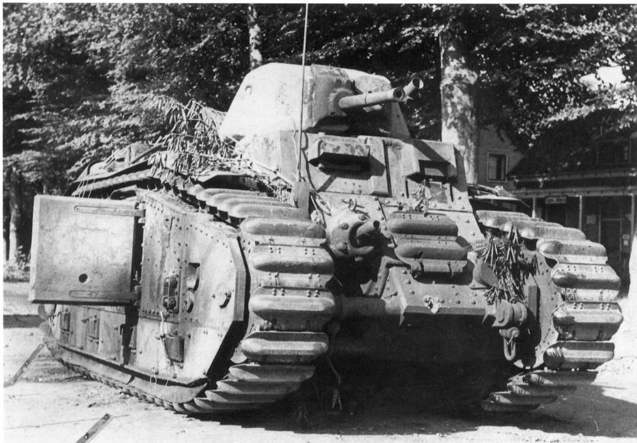
This Panzerkampfwagen B2 (F) was knocked out in Osterbeck near Arnhem, Holland, towards the end of September 1944. A old style smoke candle discharger was fitted to the side of the turret by the unit. (Bundesarchiv)
