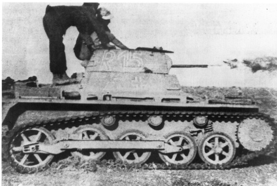
Panzer Regiment 5 created these makeshift Panzerkampfwagen I (Flamm) by installing a back-pack flamethrower in place of one of the MGs in the turrets of some Pz.Kpfw.I Ausf.As. These Flammpanzers attempted to dislodge the defenders from their concrete bunkers around the perimeter of Tobruk.
