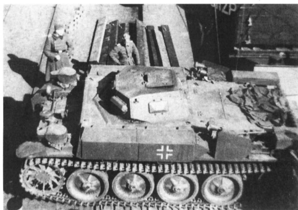
Rare overhead view of a Panzerkampfwagen II (F) – based on the Panzerkampfwagen II Ausf.D – revealing the two Spritzköpfe and the shape of the turret. (Wegmann)
