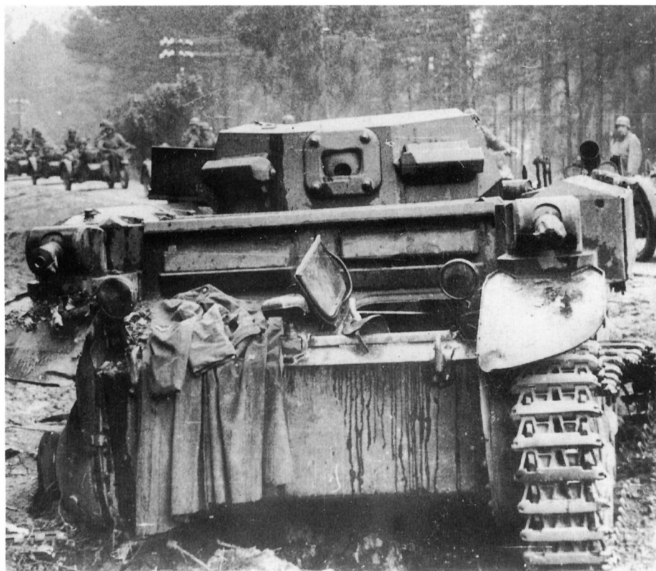
Panzerkampfwagen II (F) destroyed during the advance into Russia in July 1941. This photograph gives a rare view of the front of a Panzerkampfwagen II (F). (Bundesarchiv)
