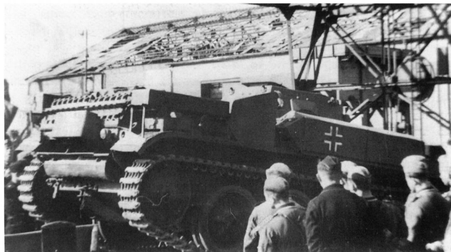
Right-hand rear of the Panzerkampfwagen II (F). A smoke candle dispenser is mounted on the rear plate, but is supplemented by three forward firing smoke candle launchers positioned behind the flame fuel tanks. (Wegmann)
