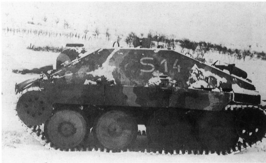
Side view of a Flammpanzer 38 captured by the Americans. These Flammpanzer were converted from 20 Jagdpanzer 38 built by BMM in Prague in 1944. The flame projector system is identical to that developed for the Sd.Kfz.251/16 with cartridge ignition. (US Official)
