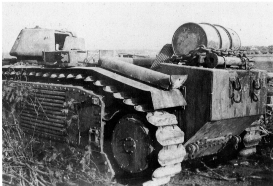
A special feature of the last series of the Panzerkampfwagen B2 (F) was the large armoured flame fuel tank added to the rear of the hull. This particular Panzerkampfwagen B2 (F) was destroyed near Deventer, Holland, in April 1945. (Tank Museum)
