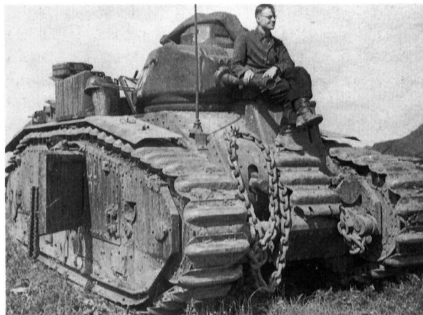
The second series of the Panzerkampfwagen B2 (F) had a new flame projector system. The projector was again mounted in place of the 75 mm hull gun of the original French Char B, but the pressure for the flame fuel was provided by an auxiliary motor. First deliveries of these conversions began in November-December 1941. (Werner Regenber)
