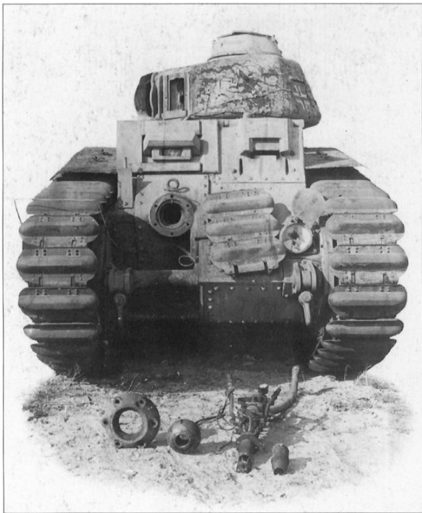
The final series of Panzerkampfwagen B2 (F) had a new ball-mounted flame projector. The fighting compartment was extended and a driver-type vision block with an armoured visor provided for the operator. This photograph shows the ball mount and projector disassembled. (Tank Museum)
