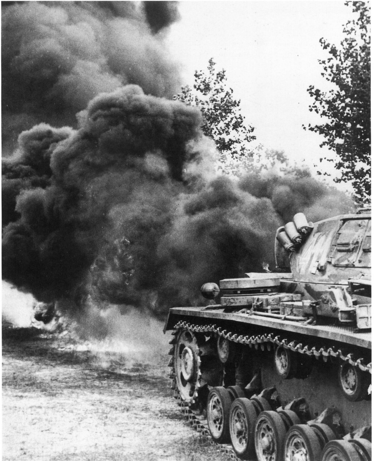
The Flame projector was designed to eliminate bunkers at a relatively short range. (US Official).
